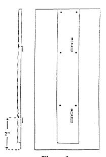
25 CL Can Shim (right) Part #495,010,10x.x3 25 CL Can Shim (Left) Part #495,010,00x.x3
